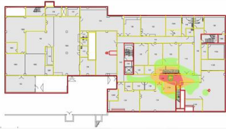
Mechanical Engineering before upgrade – inadequate coverage
